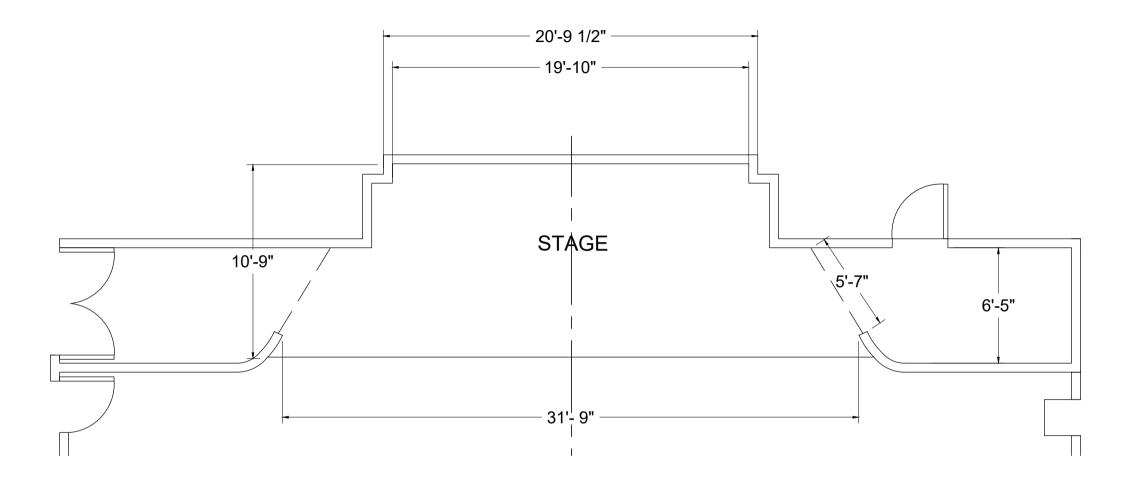
STAGE HEIGHT = 0'-9" PROSCENIUM OPENING HEIGHT = 11'-3" STAGE WING CURTAIN HEIGHT = 7'-0"
